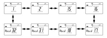
5. In sub-channel settings, after the channel is set to 17 to 32, the assigned buttons below are pressed. Pressing each of the buttons activates or deactivates the sub-channels (A, b, c or d). When a sub-channel is activated, the corresponding sub-channel letter appears on the display. If a sub-channel is deactivated, a "-" is displayed in place of the letters.
