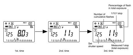
5. To clear the cumulative value, press M. CLEAR button ② or switch to another mode by turning the Jog wheel while pressing the mode set button.
