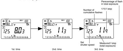
3. The ready to measure mode will be displayed for approximately 90 seconds. If the 90 second period is exceeded and the blinking mark stops, press the Measuring button () again. The measured value (f stop) of the previous time reverts to 0 and the meter is in ready to measure mode.
