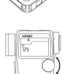
4. Press the Measuring button (4) to trigger the flash. The measured value (f stop value) will be displayed.
